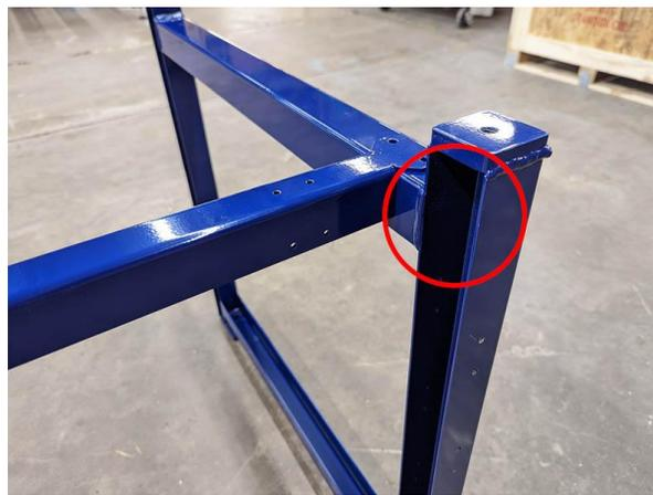
Lay two stand struts (006309 or 006310 depending on your model) across the top of the legs so the holes in the end flanges line up with the threaded holes on parts 006308. Use 8 BHSCS  $\frac{1}{4}$ -20 x  $\frac{5}{8}$ " to secure the struts, but **don't tighten them all the way**.
