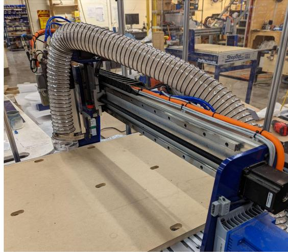
Secure the hose with zip-ties at two points along the top of the gantry. The first should be a little bit past the end of the e-chain and the second is right at the end of the gantry. The first connection should be somewhat loose, try moving the YZ-car back and forth to make sure that the hose routes accordingly.
