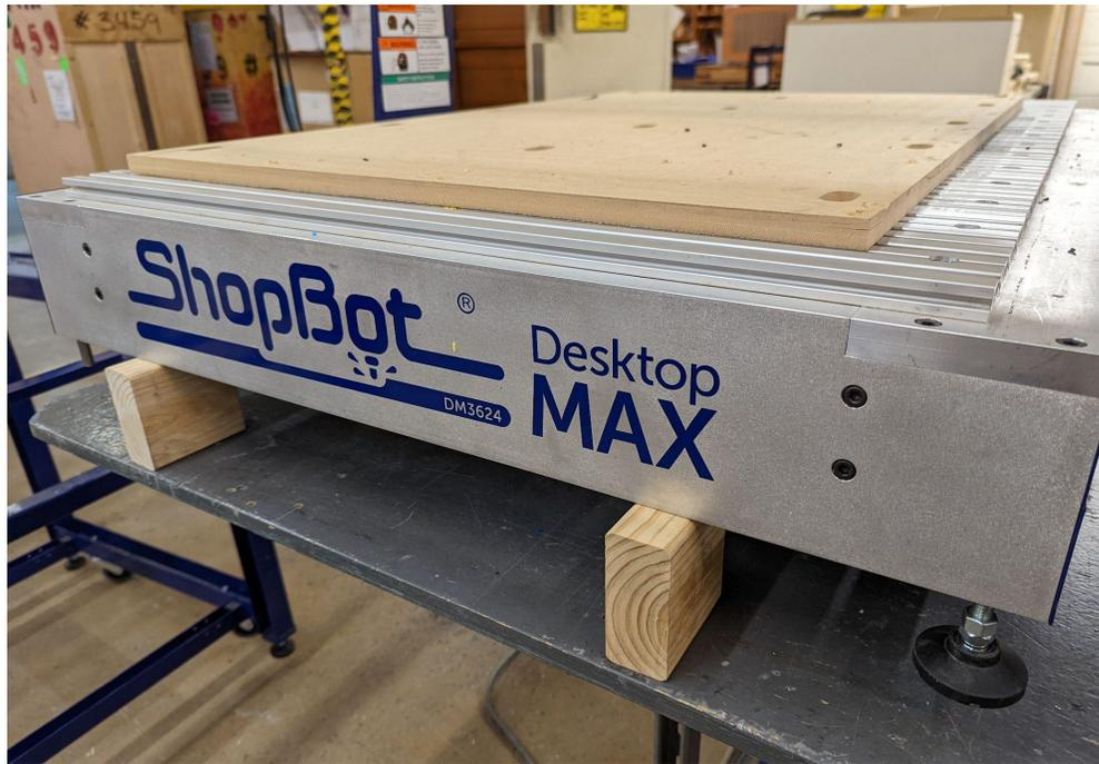
Replace the levelers with 4 Partially Threaded Studs  $\frac{3}{8}$ -16 x 2" (006380). These will be used to help line up the tool to the stand. Remove the nuts on the levelers, then screw the levelers into the threaded holes on the bottom of each leg as far as they will go. Reattach the nuts to the end of the threaded studs inside the legs.
