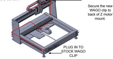
All ShopBot models have a wago connector for attaching several Z Axis Zeroing Devices. You will be using this connector to power your laser pointer.
