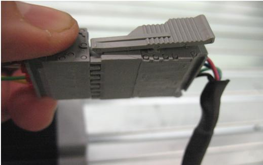
**RIGHT: both ends tightly connected**
