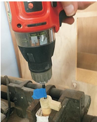
fig. 4i Drill hole into dowel end using existing hole in part #6 as a guide
