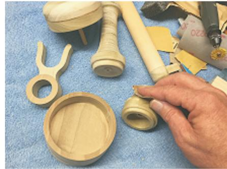
Sand and blend sections of all assemblies. (fig. 4l)
