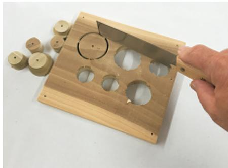
Separate the parts from boards
