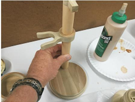
Glue dowel post into the base with tenon facing forward.
