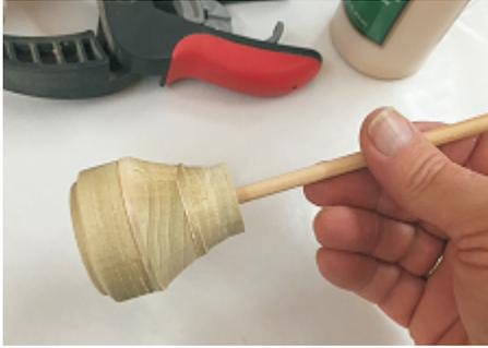
Glue the 1,2,3 sections together. Align with a scrap dowel, then remove the dowel immediately after glue-up.
