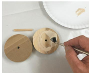
Make sure the dowel end is flush with the pocket bottom on the backside of section #5
