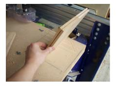
Remove the screws from the hold down. Grab the piece of wood and flip it over in the X position. Note that the edge of the board that was at X=0" will now be at X=10".
