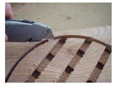
Tabs are used to hold the project to the waste material. This keep the parts from slipping during the cutting process. Simply find these tabs, score them with a utility knife, remove the project from the waste material and sand off the tabs.
