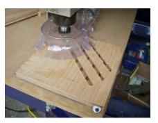
Reinstall the hold down, load the second cutting file which also includes the profile cut that removes the project from the scrap. During this cut the previous toolpath will be exposed from the underside.
