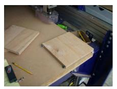
The dado is 3/16" deep into the board and should have the dado half way through the thickness of the material.
