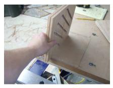
Here is a shot from another view. This is showing how the board is simply picked up, rotated and placed cut side down. Make sure the board is centered within the pencil trace marks done earlier.
