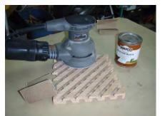
Thoroughly sand the projects surfaces with a power sander. Also use hand sand paper to knock down any sharp corners. Follow any manufacturers finishing instructions or simply rub food grade mineral oil into the wood until it coats evenly.
