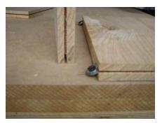
Hold down for this project can be done by using screws in each corner through the face, or by ripping a dado on all four edges of the project as pictured above.
