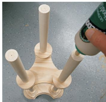
Apply glue to each dowel end, place the Top Support back onto the posts, then drive three drywall screws through the support and into the dowels. (fig. 5h, 5i)
