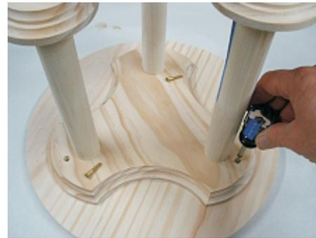
Drive the three 1" #6 woodscrews through the support and into the tabletop. (fig. 5l)
