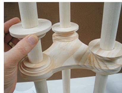
Slide the last three rings (wider side UP) onto the posts. (fig. 5d)
