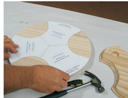
Place the taped template on the underside of the Tabletop and center it. (fig. 5b)
