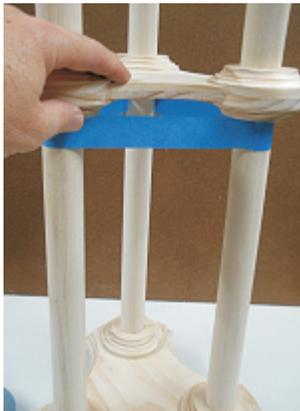
Slide the Middle Section over the posts until the bottom lines up with the tape. Allow to dry. (fig. 4q)
