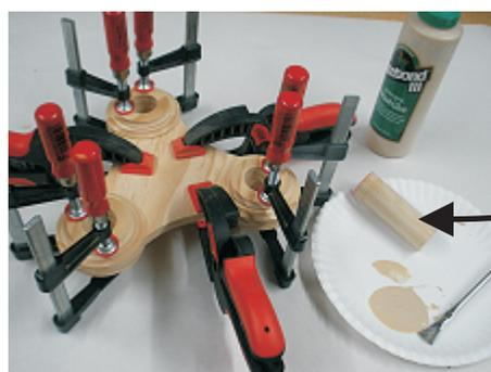
Scrap length of large dowel used for help in aligning parts
