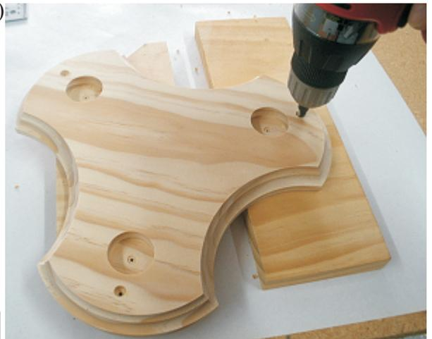
Flip the part over and drill countersinks into the flat underside at the three **inner** pilot hole locations. (fig. 3c)
