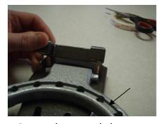
Line up the ring with the groove side up. Then apply some glue around the dowels and push the front support into place.
