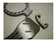
Make sure the dowels will fit in the holes nice and snug. Also make sure the dowels are no longer than 1" in length of they will push through and wreck the project.
