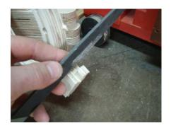
Use a hand file to shape the tenon round. If a Dremel is available it will help speed up the process.
