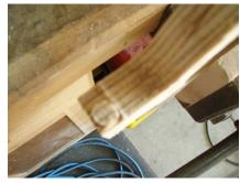
The tenons need to be round like pictured above so the hoop can turn back and forth once the whole project is glued together.
