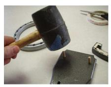
Hammer the dowels into the back piece first. This piece is stronger than the front support and putting the dowels in here first helps the front support from taking on to much stress.
