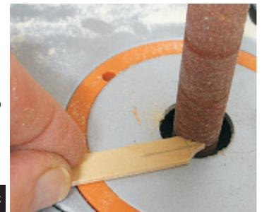
Make a "lever handle" from popsicle sticks. Glue two sticks together, then cut off the rounded end to a 0.5" length. Glue this on top of a 1" long stick. (fig. 5d)
