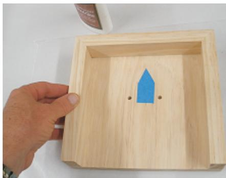
Glue the front strip to the base. (fig. 4e)
