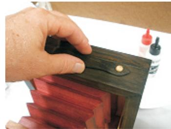
Epoxy the handle to the top of the box. (fig. 7n)
