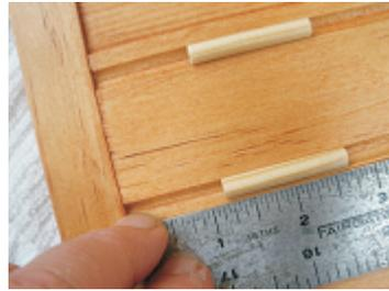
Epoxy two 0.25" x 1.5" long dowels into the slider grooves of the main base. Position them 1.1875" from the seam of the front strip. (fig. 7i)
