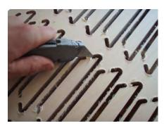
Once the file is complete, flip the work piece over and cut the tabs with a utility knife. If you try to push them out by hand it could lead to tearing out on the wood and take away from the projects appearance.
