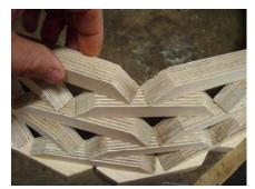
After dropping a piece into position it is a good idea to hold it there for a few seconds or simply put a little pressure on the top side of it.
