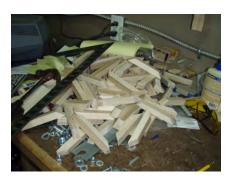
It is a good time while the handle is gluing up to go through your pieces and hand sand all the sharp edges and corners. This will allow someone from getting slivers while handling the basket.
