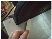
After all the pieces are removed touch the ends up to remove any tab remnants. This can be done by hand or a power sander of your choice.
