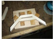
Make a jig to hold the four pieces together until the glue can set. If you do not have access to a nail gun, simply screw the jig together. Let this sit for at least an hour before moving on to further gluing.
