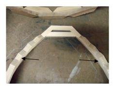
Keep an eye on the left to right spacing of each layer. Each new row will be shorter than the previous so keep an eye on the left to right balance.
