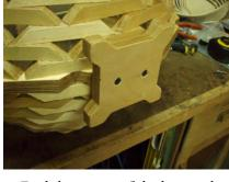
Find the center of the base and the center piece of the basket. Layout for two screws to be drilled in for extra support. Glue and screw the base onto the basket.
