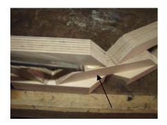
It is very easy to put extra glue onto a joint. Wait until the glue has set after an hour or so, then bring in a sharp chisel and scrape the glue from this joint. Doing this when the glue is wet tends to move the parts around.
