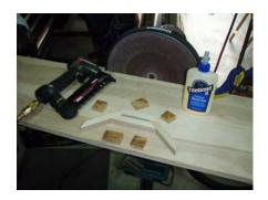
It is very important at this step to find four pieces to make up the handle of the basket. Make sure all the ends are cleaned up and at a 45degree cut.
