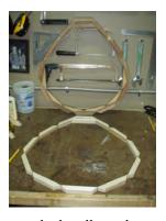
Lay out the handle with an additional nine pieces as shown above. This will become the center ring of the basket. At this point the basket should measure 19.25" tall and approximately 18.25 at its widest point. Then simply fill in the parts by eye to make the shape.
