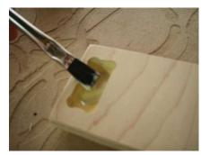
A small brush or your finger should apply the glue to all surfaces inside the mortise. This will ensure a properly glued joint.
