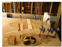
Clamping pressure should be kept on the assembly for a couple hours, this also means the chair should lay like it is pictured above during this time so glue does not run out of the dogbone corners.
