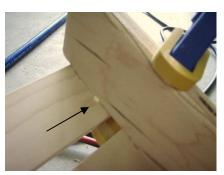
Excess glue is fine, just wipe it off with a damp towel. If you miss wiping the glue off and it dries, a sharp chisel will pop the glue heads off from your project.
