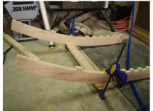
Start by gluing the back support onto the upper curved pieces. Clamp and allow glue to dry. Flipping the project over from here can allow wet glue to spill out of the dogbone corners on the mortise pockets.
