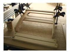
Work your way from one side to the other filling the tenons with glue, spreading the glue with a brush and applying a clamp to hold the pieces together until the glue sets up.
