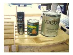
Ideally painting this chair would be easier done before assembly, it is easier to get to all of the pieces. However, it is not to much extra work to stain or paint the project after it is assembled. One can also venture into the spray finishes.
