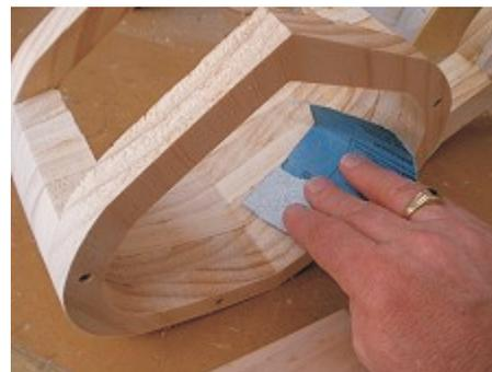
After the assembly is dry, sand the inside with coarse sandpaper to blend the sections. (fig. 4e)
