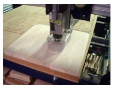
If you have a 18"x18" blank you can safely run a screw into each corner of your work piece, since you will be cutting a circle the screws will be far away from the cutter.
