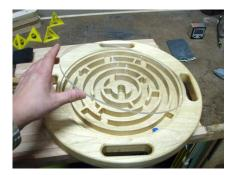
No glue is used for the glass because it will show through. Make sure the glass or plastic is clean on both sides before installing.
