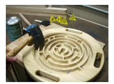
A rubber mallet may be needed to push the glass or plastic down into the groove. Try not to scuff the material.
