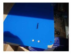
Clear plastic or Plexiglas can be used for this project. This was cut from a scrap piece, if your thickness is different then the one described in the file simply change the depth. 1/4" "O" flute from the router bit starter kit is used here.
