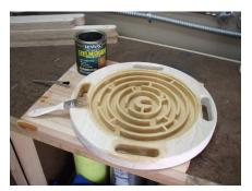
Finish the material with several coats and make sure all of the grooves are stained, once the glass is installed you will not be able to get back into this area.
