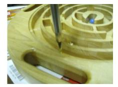
Use a small wood screw to push down into the wood material and hold the plastic in place.
