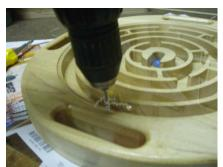
If desired, screws can be added to help keep the glass seated. Evenly space as many holes as you want and predrill the plastic or glass only.
