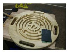
Before applying the finish it is a good idea to route all of the handles and outside edges of this project with a round over bit. This will make the project more comfortable to handle.
