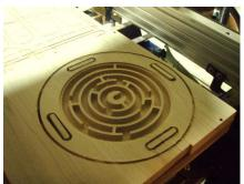
Once the piece has been cut, pop it out and sand all of the edges and faces. Make sure it is smooth for the marble to move around on.
