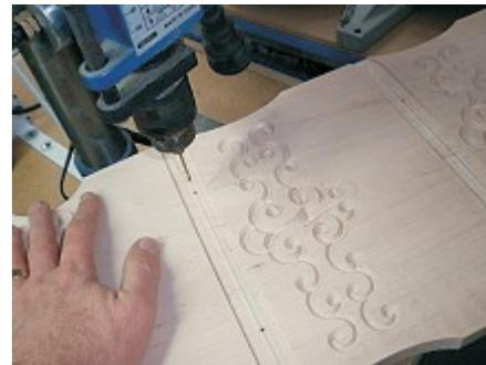
Drill six pilot holes through the board at the marks. (fig. 4e)
