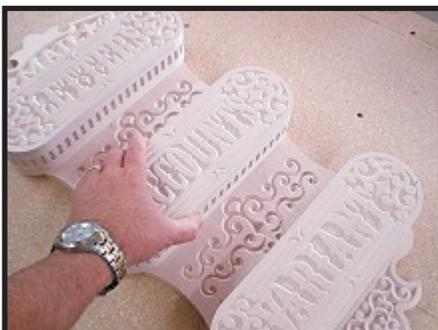
Test-fit the mail holders onto the Main Panel. (fig. 4c)
