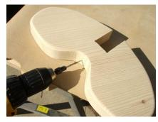
For extra strength to hold the elephants ears in place a post-Shopbot step would be countersinking a hole through the ears into the elephants head.
