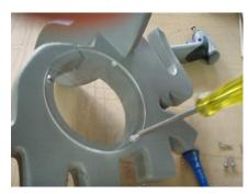
To ensure the Plexiglas is not cracked by over tightening, use a hand driven screwdriver and put the screws in by hand.
