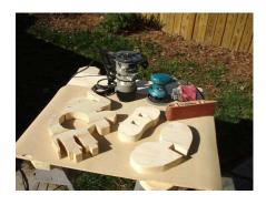
Route and sand the entire project to ones liking. Remember that this will be handled by children and should be free of any sharp corners or splintered wood.
