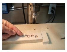
One can by wooden plugs to plug the countersunk hole or use a plug cutter to make your own. Apply glue to the plug and use a rubber mallet to fill the hole on top of the elephants head.
