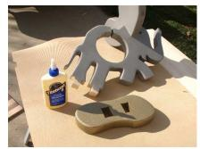
Make sure the tenons on the bottom of the elephants feet fit into the pockets on the base. Sand them if need be, just do not force and break off the tenons.
