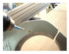
Depending on the size screw one chooses to use will depend on the pilot bit size. Make sure the proper sizes are chosen before drilling.
