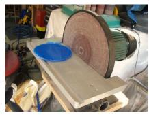
Sand off the tabs and run some hand sand paper down the edges of the Plexiglas so it is smooth to the touch.
