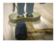
After some glue has been dropped into the pockets, use a rubber mallet to help secure the mortise and tenon joint together.
