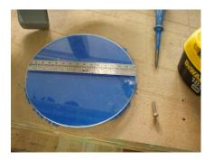
Use a center punch and a drill to layout the holes for installing the Plexiglas. This can be done on the ShopBot with a bit change, but it is quicker to do this step by hand.
