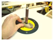
Due to the superior accuracy of the ShopBot some of the parts will be hard to fit together at first. Use a spindle sander to open up some of the pieces to fit together nicely.
