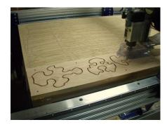
The same goes for the red oak piece, there is a toolpath file for hold down and tabs will need to be removed.
