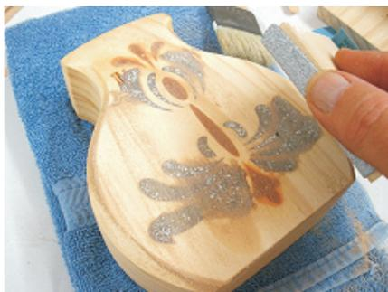
Stop sanding with 60-grit when you see the design “ghosting” through. Switch progressively to 80, 100, 120, 150, 220, 320 until the surface is completely smooth.
