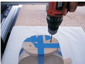
Use a long-reach drill bit to drill pilot holes for the screws through the base, and into the coin assembly. (fig. 5b)
