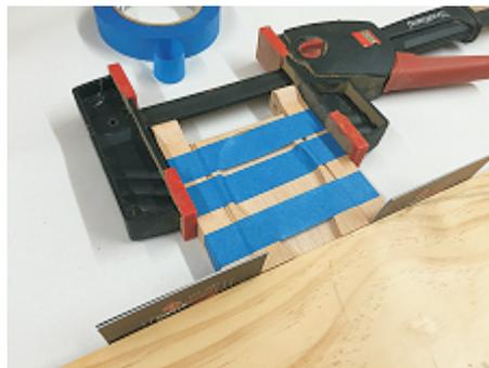
Tape and clamp the hinge arms securely in position to the sides of the main panel
