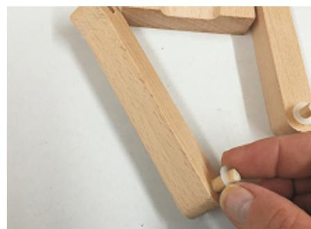
Slide one or two nylon washers onto the dowels. I used two washers per dowel because the washers were so thin.
