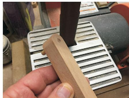
Trim and sand the excess dowel flush with the outside surface of the hinge arms.
