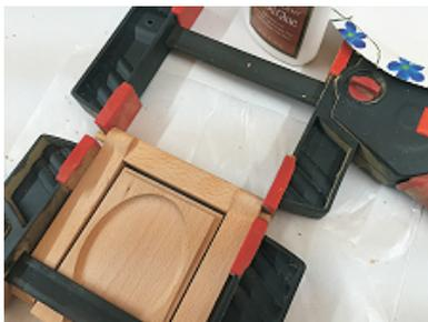
Clamp until dry, then trim and sand the excess dowel flush to the hinge arm surface
