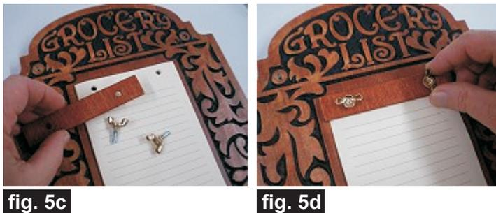
Drill pilot holes for the screw hooks at the small divot locations near the bottom and install the hooks onto the plaque. The hooks will cradle a pencil or pen. (fig. 5e, 5f)
