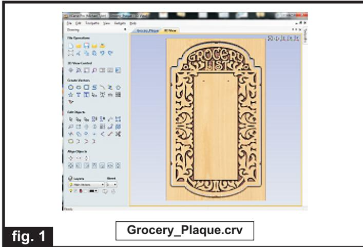
Carefully review all the toolpaths and make any necessary changes to suit your particular bits and machine. The toolpaths are currently set with feeds, speeds and pass depths that were used in creating the original sample. Please don't use them directly until you review them for your own setup.
