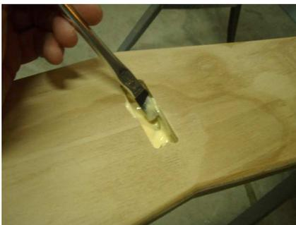
Just like before from the seat apply glue to the remaining mortises on the backrest.
