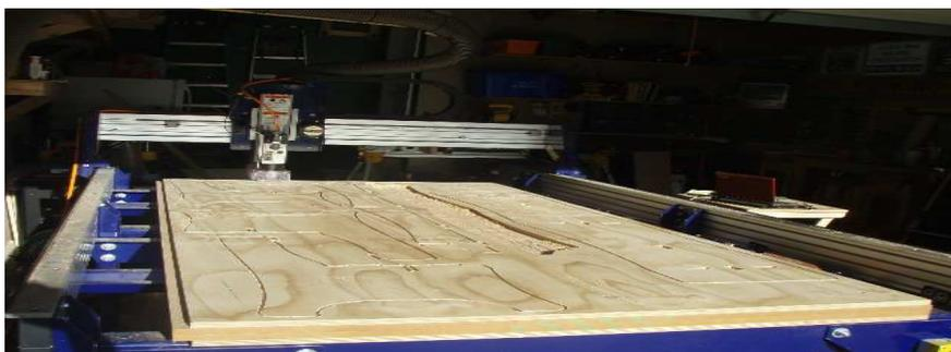
As the file starts cutting the profile of the parts make sure the cut is going all the way through the work piece and into the table surface. If you need to adjust any part of the file make sure you do not remove the hold down or you will loose position.
