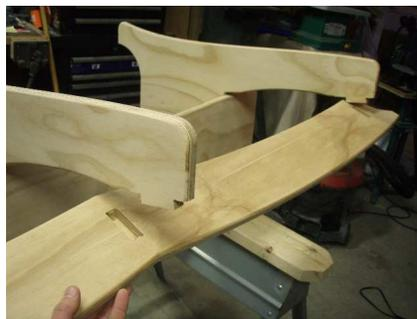
Position the bench so that the glue will not run out of the backrest during the glue drying time.
