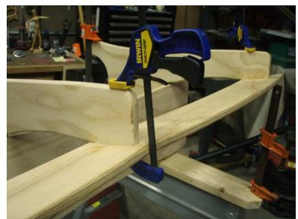
Make sure clamps are used to hold the pieces together until the glue has setup.
