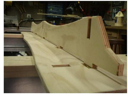
Insert the bottom stringer first. It can go either way, all of the tenons are centered to the seat. Push this down in place before moving to the next step.
