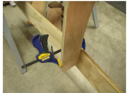
For alignment purposes the backrest is dry clamped into place with no glue. This will help hold the project square while the glue sets up from the previous assembly.
