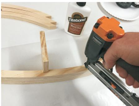
You can use drops of CA glue or pin nailer to tack parts after alignment
