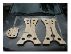
There will be four sets of stools consisting of two sides and a foot rest. Lay them out like the picture above before you are ready to assemble.
