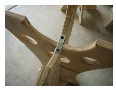
Make sure you install the strapping over the two gaps in the wood. You want to pickup the piece that is flimsy and hold it to the other leg.
