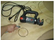
Tabs are used to hold the pieces in place while they are being cut. Simply flip the board upside down to expose the tab and push a utility knife through them removing the part. If you have access to a RotoZip this will speed up the process.
