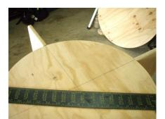
Using a straightedge draw lines from the center of one leg to the center of the next. You are creating a layout line to run screws in, it can just be eyeballed.
