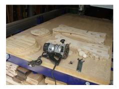
After the tabs are removed and the edges are sanded it is not necessary but adds a lot of eye appeal to route all of the edges with a 1/4" round over bit.
