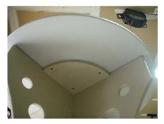
Run three screws into each corner section. Note if you are using 1 1/4" screws and you run them in to deep they can pop up and through the top. Just run them flush with the bottom board.
