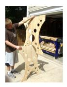
To start assembling the table simply hold the groves over each other and push the side pieces together.
