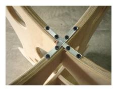
Lay the two brackets on as pictured above. Spanning the joint with these brackets really stiffens up the table.
