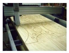
A hold down file is provided for this project. This will locate the screw locations prior to loading the cut file. Make sure that the proper hold down file is used for the correct board you are cutting.
