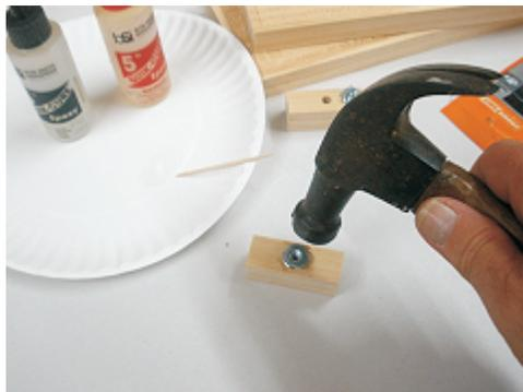
Glue the screw mounts to the interior side panels. Glue them just below the top surface of the sides so the T-nuts won't interfere with flush glue-up of the top panel later. Clamp until dry. (fig. 4b, 4c, 4d)
