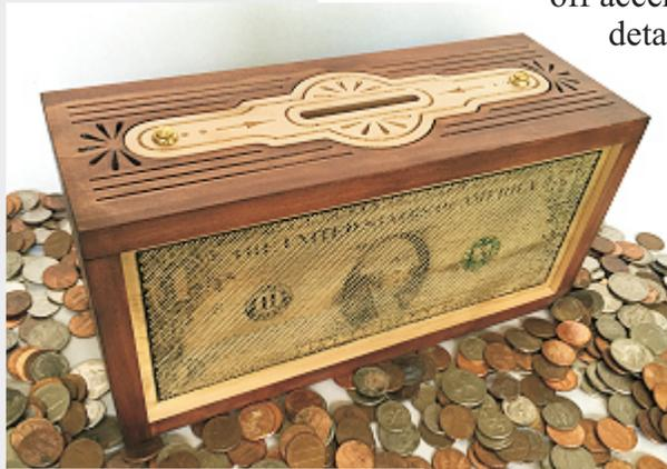
The coin access panel is a decorative v-carved inlaid part sized appropriately using the convenient Inlay Toolpath feature with automatic compensation for the tool radius in VCarve Pro (and
