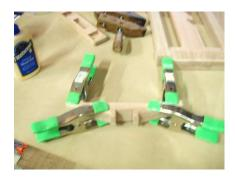
Spring clamps have enough pressure to keep the parts held together. Make sure the pieces are as flush as possible with each other to cut down on sanding time after the glue is set.
