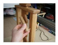
Push the other end onto the dowel and flush that end as well.
