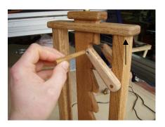
Make sure the ratchet lock is positioned like it is in the picture before inserting the second dowel. Failure to do so will prevent the lock from working properly.
