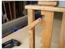
Install one side and flush the dowel with the lock. Your particular dowel length can be measured by using the thicknesses of your parts.
