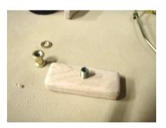
Using a hand drill make the hole just smaller than the diameter of the threaded nipple. This way one can screw the nipple into the wood and use a little epoxy if necessary to hold in place.
