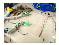
Since one end of the cord comes installed, make sure you run the cord through the foot with the groove. Also make sure there is approximately 3: of cord at the top of the part.
