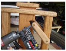
Using a small pin nailer plug a couple pins into the dowels to keep them from falling out. If no pin nailer just dab a little glue in the hole and it will hold just fine.
