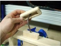
Apply glue to the underside of the top piece and slide it into place.
