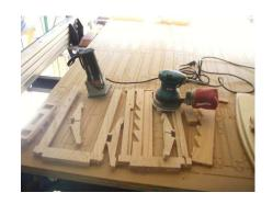
Once the parts have been cut take some time to sand all the edges and faces thoroughly. A routed edge on the outer edges will add some character to the project.
