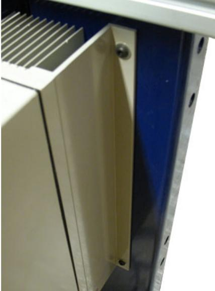
Use two holes down the right side of the VFD and mount the VFD to the middle leg of the ShopBot using the 10-32x7/8" button heads, #10 flat washer, and #10 nut. Depending on the vintage of machine, there may not be holes down the middle of the leg (three holes). A drawing is included at the back of this document for locating these holes for retro-fit purposes.
