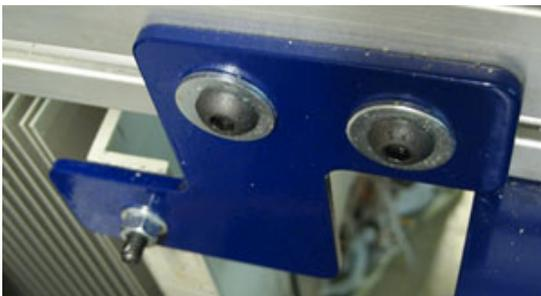
Slide the upper control box bracket so that its mounting hole aligns with the mounting hole of the VFD.
