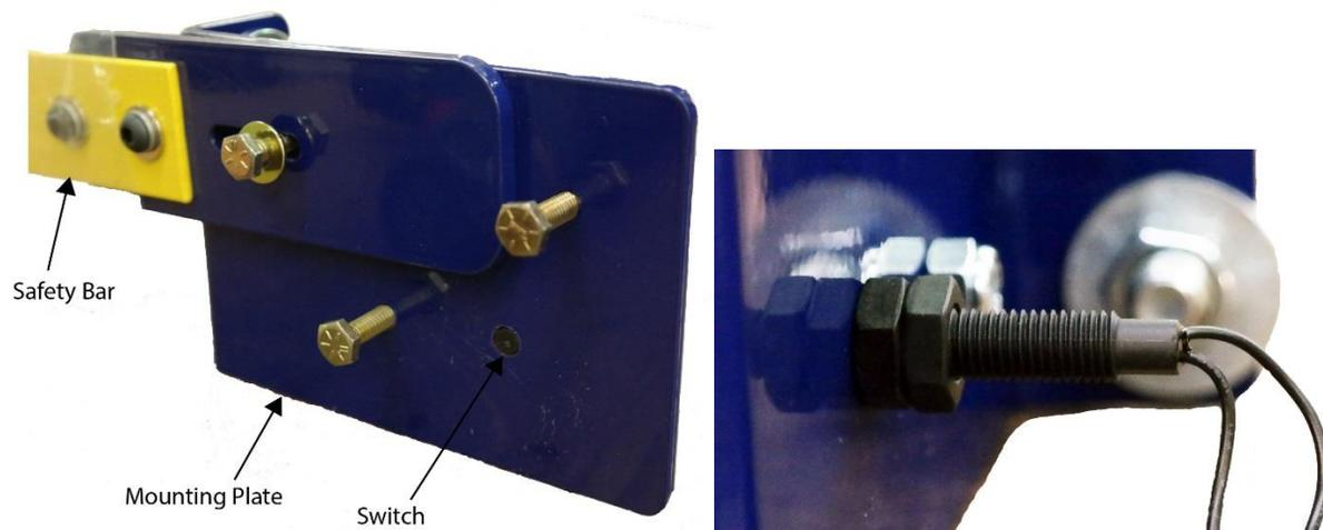
Ensure switch cable is running *under* the table between the two bars, not on the outside or over the top, and mount the two assemblies onto machine using **(8) 1/2" x 1-1/2" hex bolts, (8) 1/2" lock washers, (16) 1/2" flat washers, and (8) 1/2" hex nuts**. Orient the assembled bar so the bar can hang down vertically when unlocked. Use the enclosed bolts, washers, and nuts to mount them to the legs as shown below.
