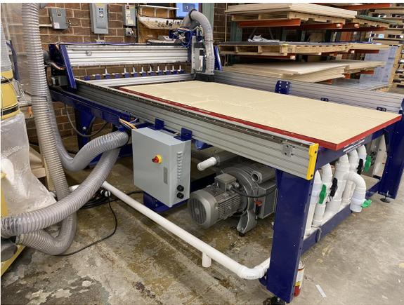
Figure 1: Standard Control Box mounted on 96x48 tool.
