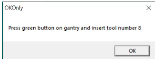
If any of the tools 1-7 are currently loaded into the spindle, the tool will be dropped off at the toolbar. The machine will then move the spindle to a central location on the table that should be easy to access by hand.
