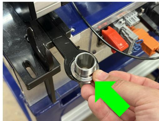
Next, select a collet sized to match the bit that you want to insert into the toolholder. Drop the collet into the toolholder with the longer, tapered end pointing down into the toolholder cone. Place the collet nut on top of the collet and give it a few turns by hand to get it started on the threads of the toolholder.
