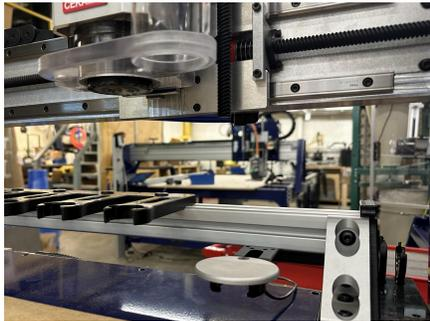
The machine will move the spindle back towards the toolbar and come to a stop above the first tool clip on your toolbar. Once the machine comes to a stop above the first tool clip.
