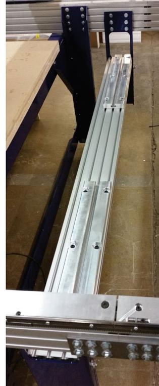
After the carriage bolts are in place, adjust the beam left-right so that it is an equal distance from the hanging bracket on either end. There should be about a  $\frac{1}{4}$ " gap.
