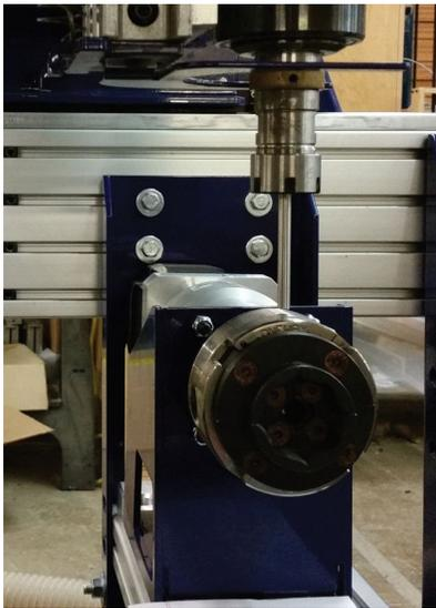
Use the same technique to align the indexer vertically, by bringing the drill rod down from above rather than from the side.
