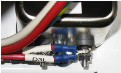
Remove nut from bottom of the Filter. Match the new wires to the existing ones: red goes with red, white goes with white. Put the open ring of the wire connector onto the screw post and tighten the nut. Make sure wires are tight and secure.
