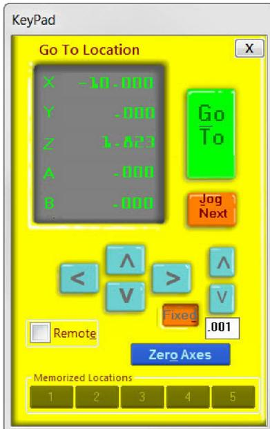
Identify the location where the z zero plate can be laid flat and move the spindle over this location. Note and record the X or Y offset from the zero position - in this example -10 inches. This will be programmed into the software later.
