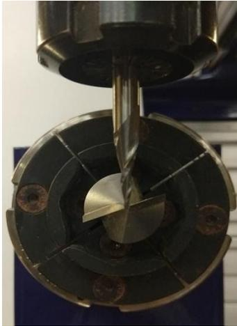
Center the spindle, as close as possible, relative to the headstock. Once in place, use the fixed mode on the keypad to make fine adjustments.
