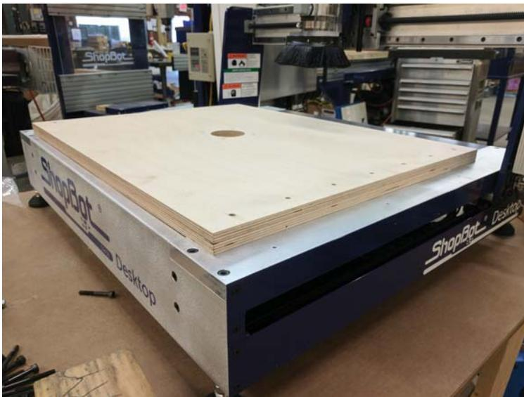
Next, install the included vacuum plenum. The plenum is a piece of 3/4" plywood with channels cut in it to allow airflow for the vacuum system to work. It sits directly on top of the plywood deck. Make sure that it is flush on all edges with the deck and that all the bolt holes line up as well as the center hole(s) for the vacuum piping. It is possible to install this piece backwards, but the large hole(s) for the vacuum will not line up.
