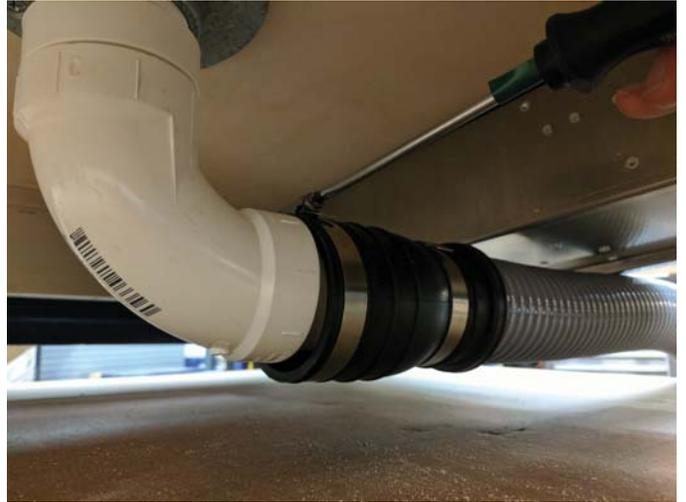
Make sure the hose is routed under the cutout section of the frame, and then lower the machine down carefully. make sure there is enough clearance under the machine for the hose. If the hose is being crushed by the machine, raise the leg levelers a bit more.
