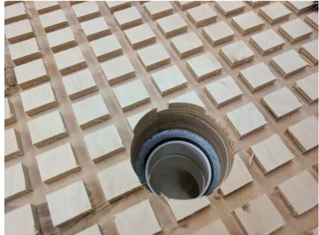
Once the vacuum plenum and deck are both in place, bolt them in place using the included M6x50 Socket Head Cap screws and a 5mm allen wrench. Do not tighten any of the bolts fully until all the bolts are started, otherwise it is very difficult to install.
