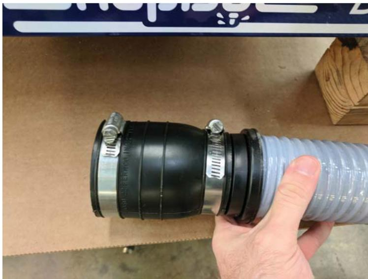
Route the hose with the rubber coupler under the machine from the rear. Place the rubber coupler over the PVC pipe and tighten in place with a flathead screwdriver.
