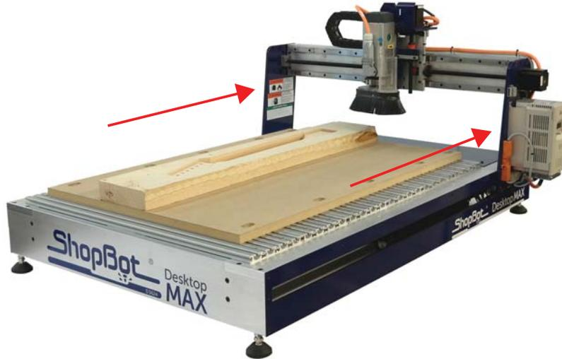
If necessary, remove the bolts holding the aluminum deck in place using a 4mm allen wrench. There are 24 bolts on the MAX and 16 bolts on the Desktop. If a spoilboard is installed on the aluminum decking, it can stay attached and does not need to be loosened.
