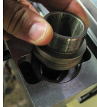
Press and hold the button on the side of the tool chuck. Rotate the tool holder until it seats into the chuck. Release the button to lock it into place.
