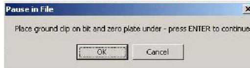
When the bit is located over the area needed to set as zero, type "C2" ("Zero Z-Axis w/ Z zero Plate").
