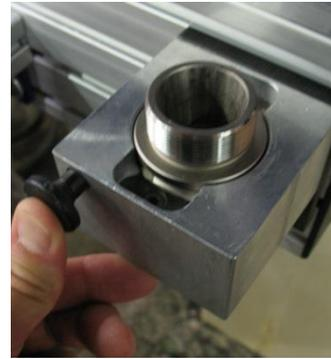
Snap the collet into the collet nut and thread the assembly onto the tool holder. Ensure the collet is the correct size for the bit needed.
