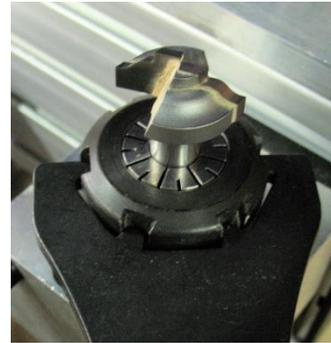
Press the button on the tool chuck to remove the tool holder from the tool chuck. Remove the tool holder from the tool chuck.
