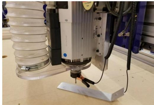
Note that the Z offset is reset to the Z home position any time the C3 routine is run. To permanently change the Z home position, refer to the Get plate offset (CN73) section of this document.
