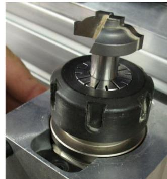
Tighten the collet nut to 100 ft/lbs with the ER32 spanner wrench.
