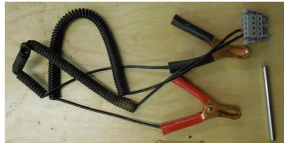
The red calibration clip will be clipped to the bottom of an empty tool holder as it is moved through all of the clip positions.
