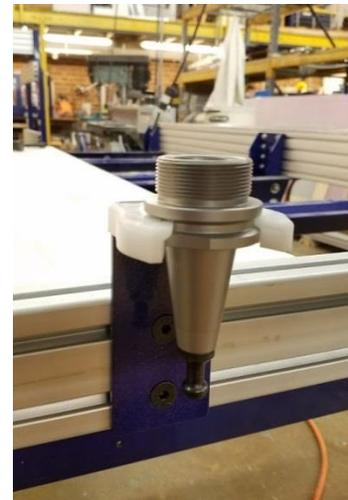
Place the black grounding clip on the tool holder in the spindle.
