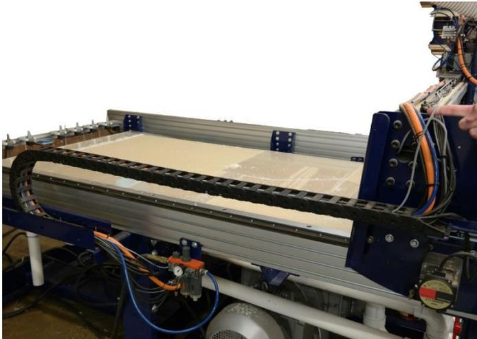
Run the ferruled side of the 3-conductor 30' ATC cable from the pneumatic manifold through the Y and X cable carriers and into the control box.
