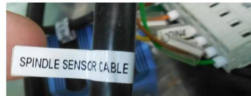
Find the female Wago connector on the board identified as "spindle sensor cable." Connect the male Wago connector into the ATC interface board.
