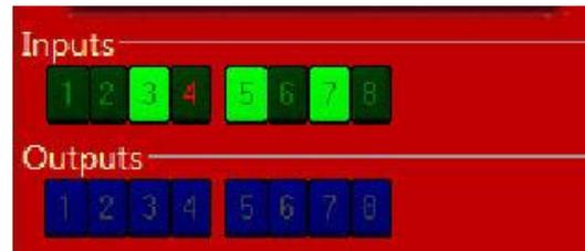
In keypad mode (K), move the Z-axis into the proximity target using “Page Up” on the keypad. The proximity switch will have a red LED lit until it comes across the proximity target, when it will turn off. Moving off the top of the target should cause the LED to come back on. This should also be evident in the ShopBot position screen when looking at input “5”. Input “5” will appear green until the target is hit then the input goes black.
