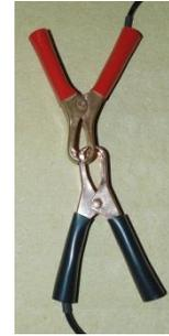
Touch the calibration clip (red) to the grounding clip (black) and make sure that input “1” lights up green on the ShopBot position screen.
