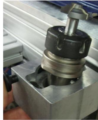
Place the loaded tool holders into the desired clip locations.
