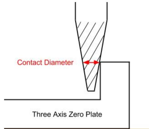
While the routine is running, make sure to hold the plate firmly in place in order to get an accurate measurement. The routine will contact the right side ledge on the inside, then on the outside, and will display the calculated contact diameter. Once you have the contact diameter, simply enter it when prompted at the start of an inside or outside corner zeroing routine.
