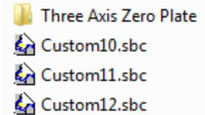
Open SB3. Click on the **[C]uts** menu. The inside and outside corner zeroing routines now appear in your list of custom cuts (see right), along with a routine for calculating contact diameter that will be discussed later (see *Using a Tapered or V-bit*, p6). The routines can be opened by clicking on them here, or by typing **CN**, then the routine number (in this case 10, 11 or 12).
