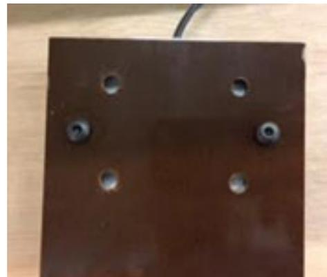
Users retrofitting an ATC purchased before 07/01/16 will need to install a replacement phenolic block (Part number 003547) in order to mount the Plate directly to the tool rack.
