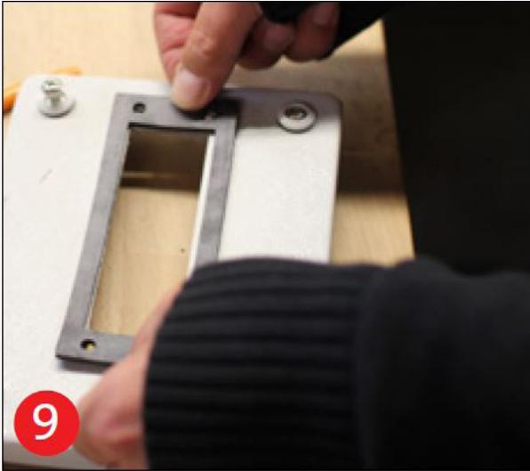
Tape the gasket around the wall cut-out
