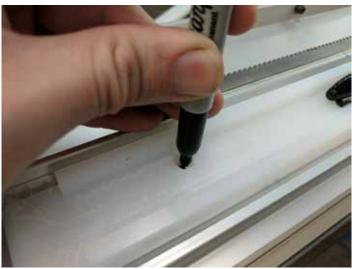
After marking, remove the upper support track. Using the provided 5/32" drill bit, drill all seven mounting holes. The hole only needs to go through the first layer of the extrusion, which is about 1/8" thick.
