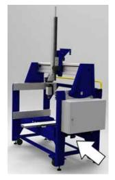
The Powerstick engages with the X-axis motor mounted underneath the deck. The motor can be engaged or disengaged using the Cam Handle located on the lower right side of the machine (shown here on a 5-Axis tool).
