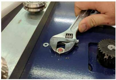
Then turn the proximity switch until it is raised above the surface of the deck as shown. The wire for the switch may need to be removed termorarily to allow the switch to turn.
