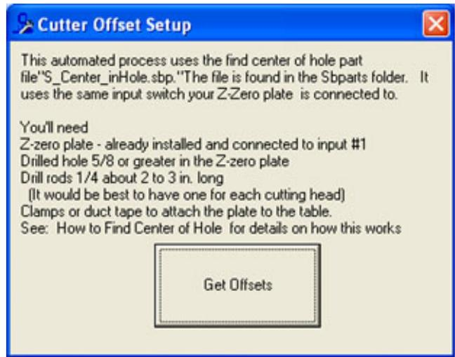
Follow the directions on the software. Center spindle #1 and click OK. If the drill rod is not in the center of the hole in the Z Zero plate, use the KeyPad to position it by clicking Yes when asked. Press Esc to close KeyPad and continue.
