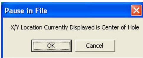
When the designated drill has pulled up, a window will open stating that the current XY location is the center of the hole. This information will be stored within the my\_variables.sbc file automatically at the end of the file.
