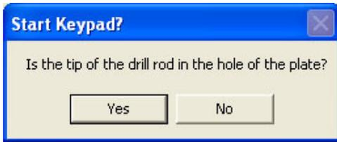
The KeyPad will close and a confirmation window will ask if the drill rod is in the hole of the plate. Click Yes if this is true and the centering routine will start. The 1/4" drill rod will start moving in the positive X direction and touch the plate. The 1/4" drill rod will move in the negative X direction and touch the plate.
