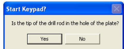
The 1/4" drill rod will first move in the positive X direction and touch the plate, then into the negative X direction and touch the plate, centering the drill rod in the X-axis. The process will repeat for the Y-axis.
