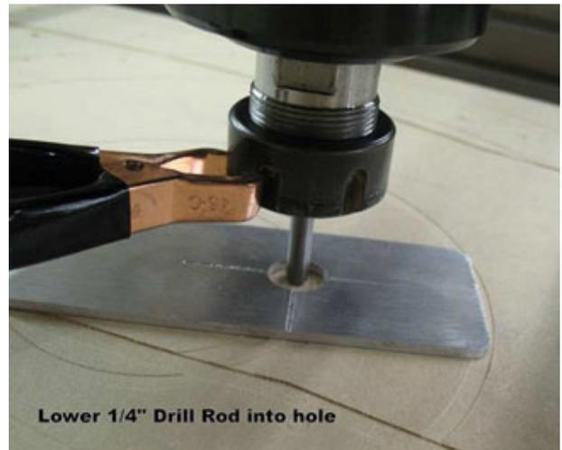
Click Yes to confirm whether the drill rod is in the hole of the plate.
