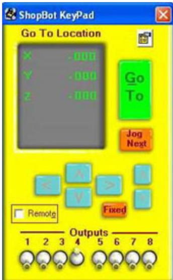
Use the arrow keys to move the primary head over the hole in the plate and then down into the hole. Be careful not to touch the table - this could cause the drill rod to drag and possibly give a misreading or loss of position. When the drill rod is in the hole, hit Esc.
