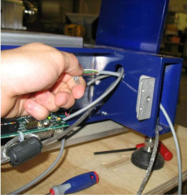
Take the loose end of the indexer wire and route it through the hole in the side of the frame.
