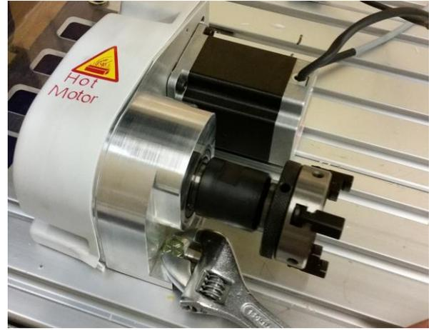
**Tightening the screws on the headstock**
