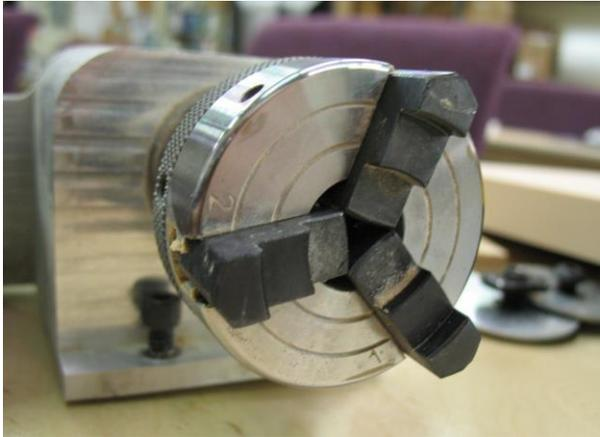
**Chuck jaw configuration: gripping inwards**
