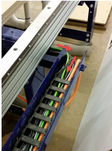
Create slack in the cables by clipping cable ties and pulling out slack, starting from the control box.
