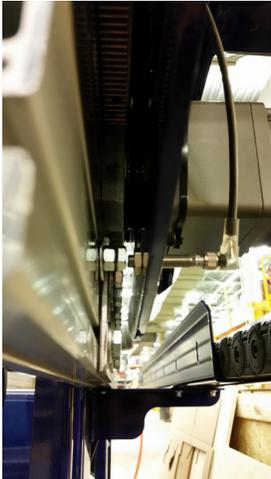
Bring the gantry back, making sure that there is about 1/16" of clearance between the end of the proximity switch and the target. Adjust as needed.
