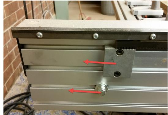
Use the provided t-nuts and gusset plate to attach the extrusion to the end of the table as shown. Make sure that the top of the extrusion is flush with the existing table sides. The gusset plate should go on the outside.
