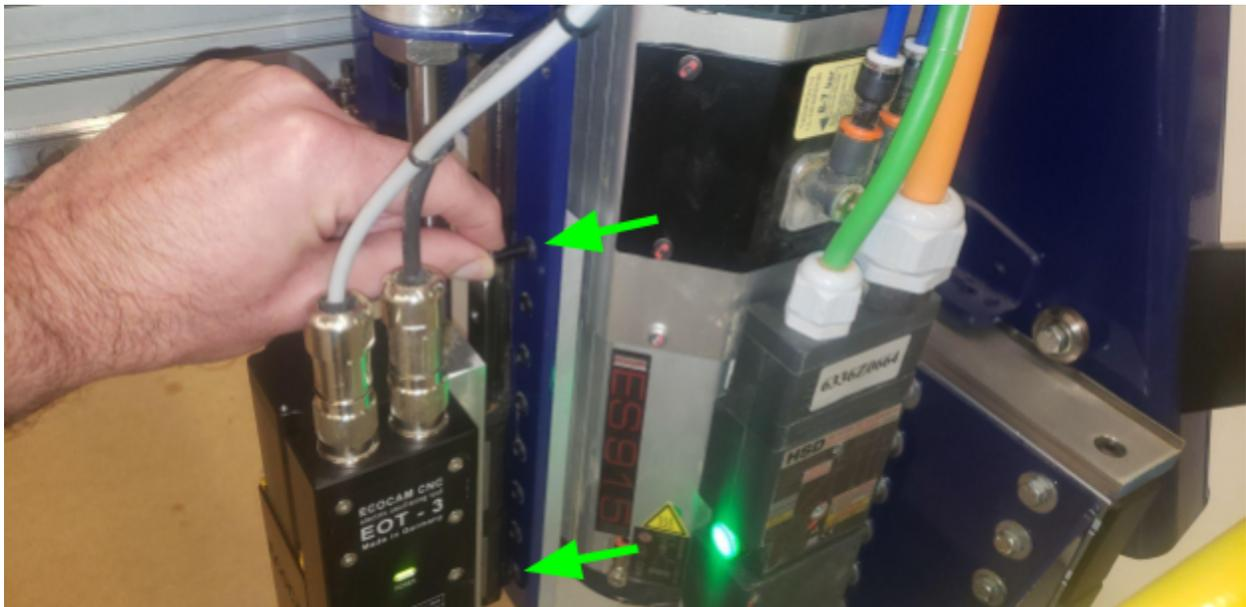
Using the four M5 HCS that were included with the hardware, mount the knife assembly to the side of the mounting adapter plate. Use the top holes and bottom holes. You will need to move the knife up and down to have full access to the holes to be able to insert the bolts and tighten them.
