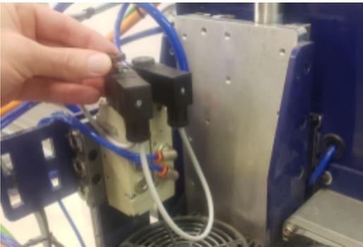
Connect the solenoid cables by sliding both connectors onto the stems. The black connector with the single gray cable slides onto the stem that corresponds with the two blue air hoses. The black connector with two gray cables slides onto the stem that corresponds with two silver plugs. Place the connectors on so that the gray cables are facing down. Secure in place by replacing the round threaded caps you removed in the previous step.
