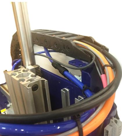
Run the three cables and blue hose into the Y and X e-chains. The three gray cables go to the control box, and the blue hose goes to the manifold.
