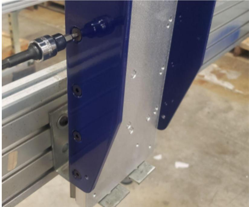
Locate and remove the bottom four flat head bolts that are on the left side of the Z plate.
