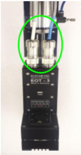
Locate the two connector ports on the front of the knife. Plug the connector with the white heat shrink into the port on the left, and the one with blue heat shrink to the one on the right.
