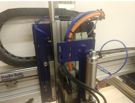
Secure all the cables and hoses using zip ties.
