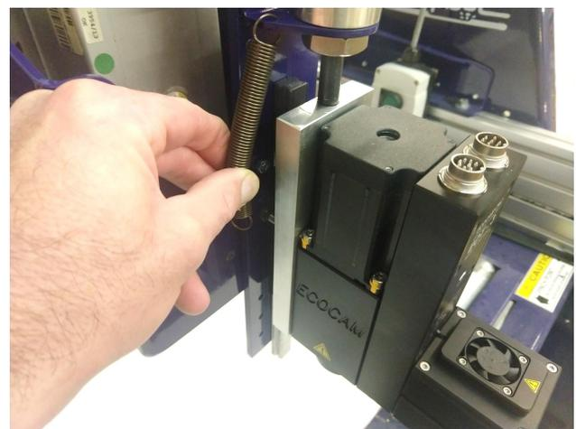
There are a few mounting heights that can be selected. The ideal mounting height depends on the length of the knife blade and the cutting length of the router bit. Select a mounting height that will place the end of the blade in a location where it will not drag on the material when it is retracted and the router bit is at full cutting depth, and allows it to reach the material when fully extended.
