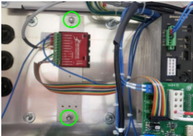
Align the two holes in the mounting plate with the two bolts. Make sure the green terminal block on the driver is on the left side. Place the two washers and nuts back on the two bolts, and tighten down completely.
