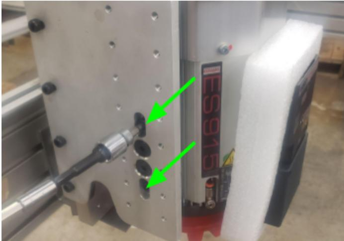
Using the other two M6 bolts that came with the knife, loosely attach the adapter plate to the two threaded holes in the side of the spindle. You may need to loosen the two flat head bolts used for the small space plate to get the holes to align. Make sure to retighten these once you are done.
