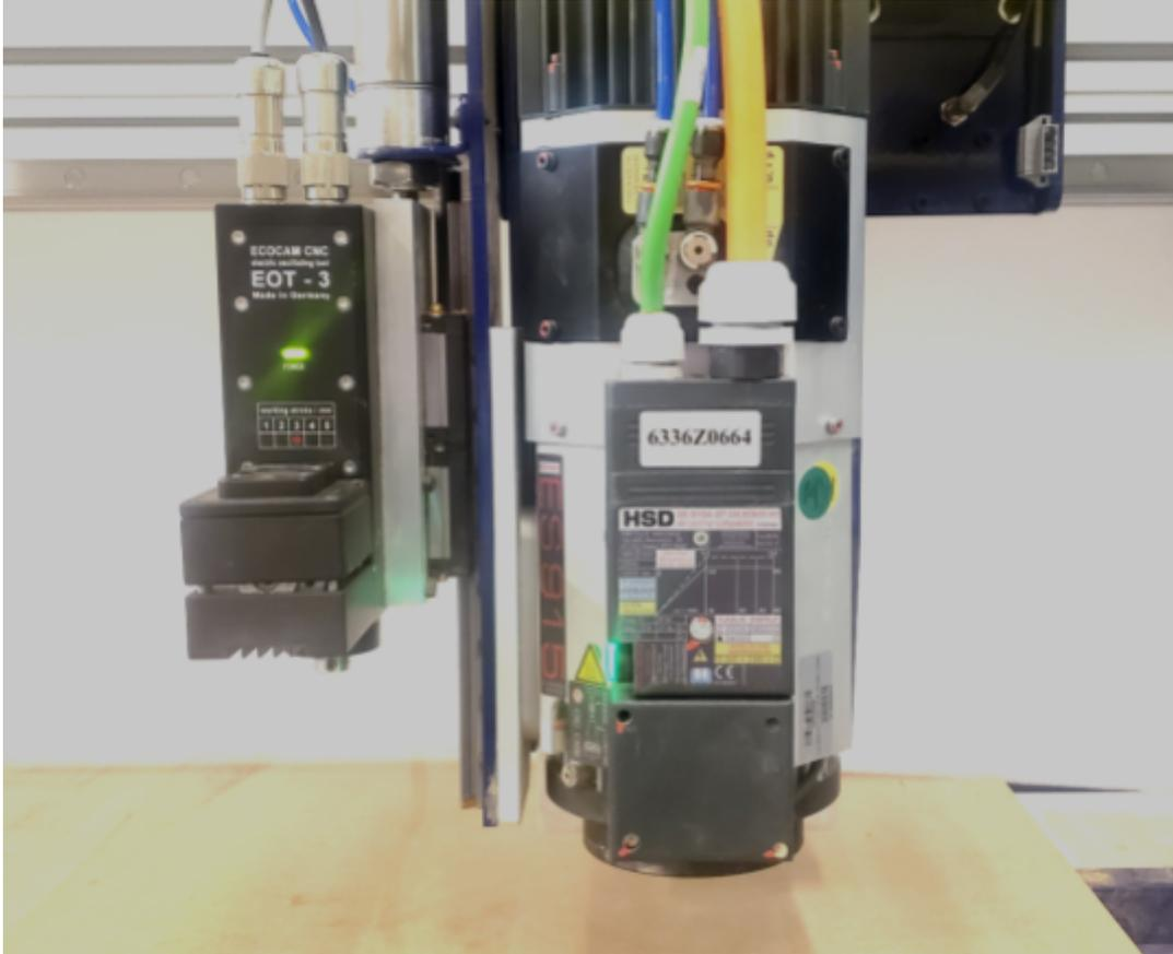
**Note:** It is important to remember that because the knife is mounted on the side of the spindle, you will lose roughly 8 inches (200mm) of travel in the Y direction.
