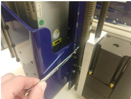
Because of space constraints the most effective tool is an 8mm open ended wrench for tightening the four M5 bolts.
