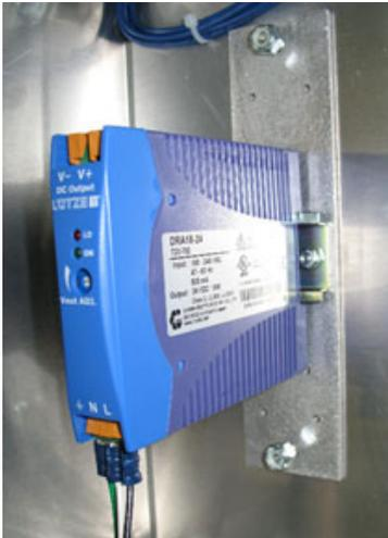
Snap the 24V power supply to the DIN rail mounting bracket.
