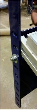
Attach the cross beam using carriage bolts, washers and nuts. For the 6" indexer, the 3rd slot from the top is typically ideal; for the 12", the 7th slot from the top. DO NOT TIGHTEN BOLTS - just thread them by hand.
