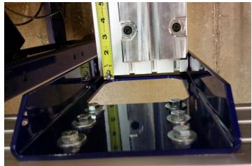
Use a 9/16" wrench and tighten the two nuts farthest from the table legs first, to pull the extrusion to one side of the hanging brackets, then tighten the other two nuts.
