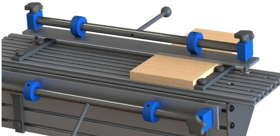
3. Slide the vertical board roughly into place and repeat the same process to tighten the clamp.
