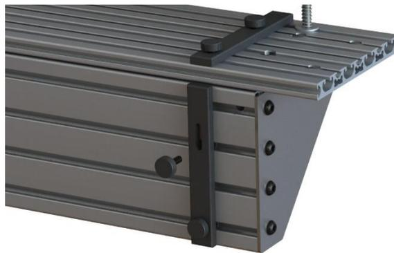
3. Reference the material you want to cut to figure out what angle to set the fence at. Slide the top knob from side to side to adjust and tighten both to set the position. Clamp the material.
