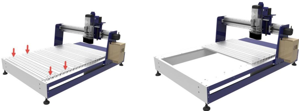
Place the jig assembly into the Desktop where the decking was just removed. Secure it to the frame using 4 of the M6-1.0x10mm button head cap screws that held the aluminum deck pieces in place. Push the clamp up against the remaining deck to make sure it is square. Then tighten down the screws, two on each side.
