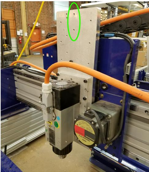
The dust hose mounting bracket attaches to the two bolt holes at the top center of the Z-axis extrusion.
