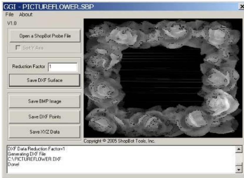
To create a DXF comprised of lines between probe points (creates a mesh of the surface of your object), press the **Save DXF Surface** button and choose a destination file name and location. This is the best option for creating a file to edit in a 3D CAD/CAM program.
