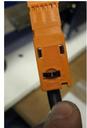
To test the router, turn on the machine and the router's main power switch. Open the ShopBot control software and set it to Move/Cut mode. Then type [K] to open the keypad move command window. With this open, click the output #1 toggle switch at the bottom of this window. The router should start up. If not, verify that the orange cable is firmly plugged in and that the router's power switch is on.
