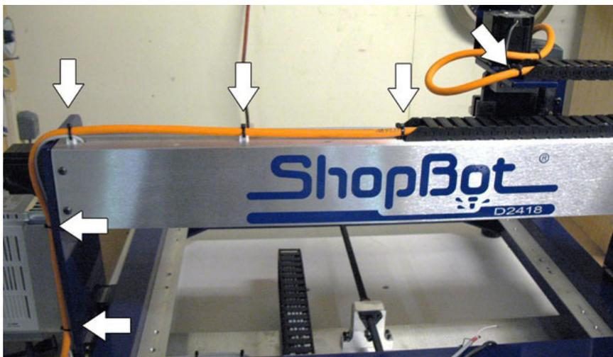
Cut any existing wire ties at the tie-down points, and use the new ones included in your hardware kit to secure the power cord along with the other links. Then close the e-chain links.
