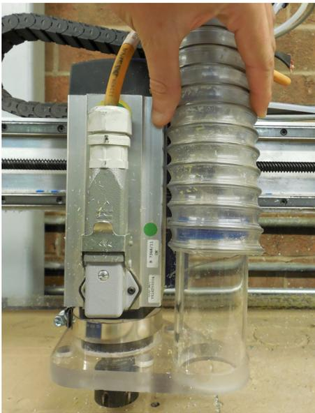
Move the spindle to the bottom of its Z travel, and overlap the hose 1/2" at the top of the plastic tube on the dust foot (blue on top of the dust foot tube is only there to enhance visibility).
