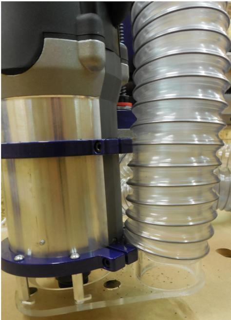
Move the router to the bottom of its Z travel, and install the hose so that it bypasses the first router mount and rests on the top of the second router mount as shown.
