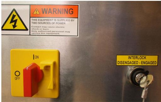
The spindle lockout switch on the front of the control box (All PRS models built after 2012) must be set to ENGAGED in order for the spindle to run. Use the key that came attached to one of the collet wrenches.
