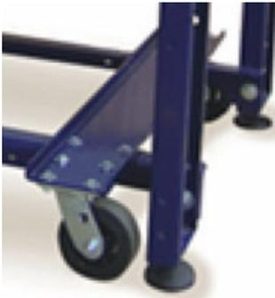
Machines with casters: Once the machine is in position, lower the leveling feet until the casters are raised off the ground again.
