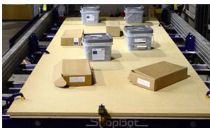
Place clamps and heavy objects onto spoil board to help glue cure.
