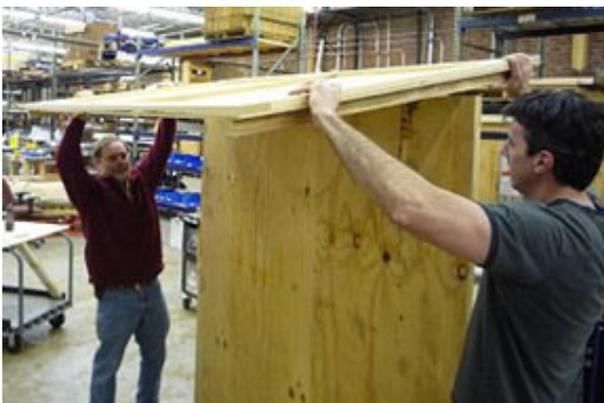
Remove screws from top edge of crate and lift/slide off top. Carefully remove crate sides by unscrewing edge brackets and freight gussets.
