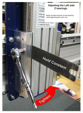
After adjusting the eccentric bearing to the proper tension as instructed above, hold the position of the bearing constant with the flat bar wrench while using a 13mm socket wrench to tighten the outer nut.
