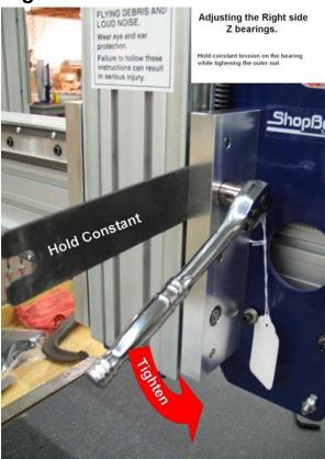
It will probably be necessary to remove the Y-axis motor to tighten the nuts on the right side. Use a 3/16 hex key to remove the Y-axis motor. After adjusting the eccentric bearing to the proper tension as instructed above, hold the position of the bearing constant with the flat bar wrench while using a 13mm socket wrench to tighten the outer nut. Reattach and engage Y-axis motor.
